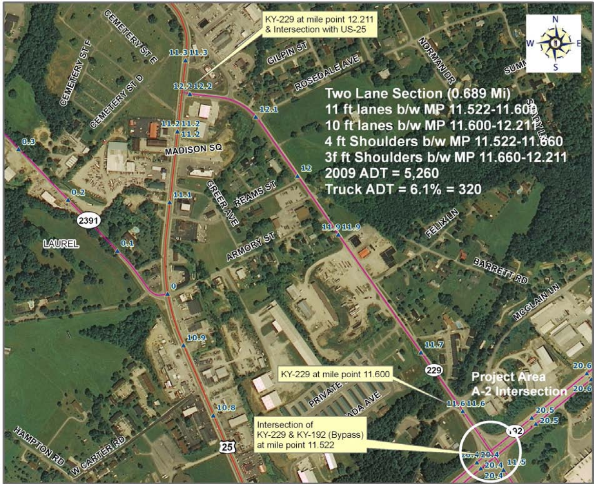
Figure III-8: Section 3 – KY-229 (from MP 11.522 to MP 12.211)
