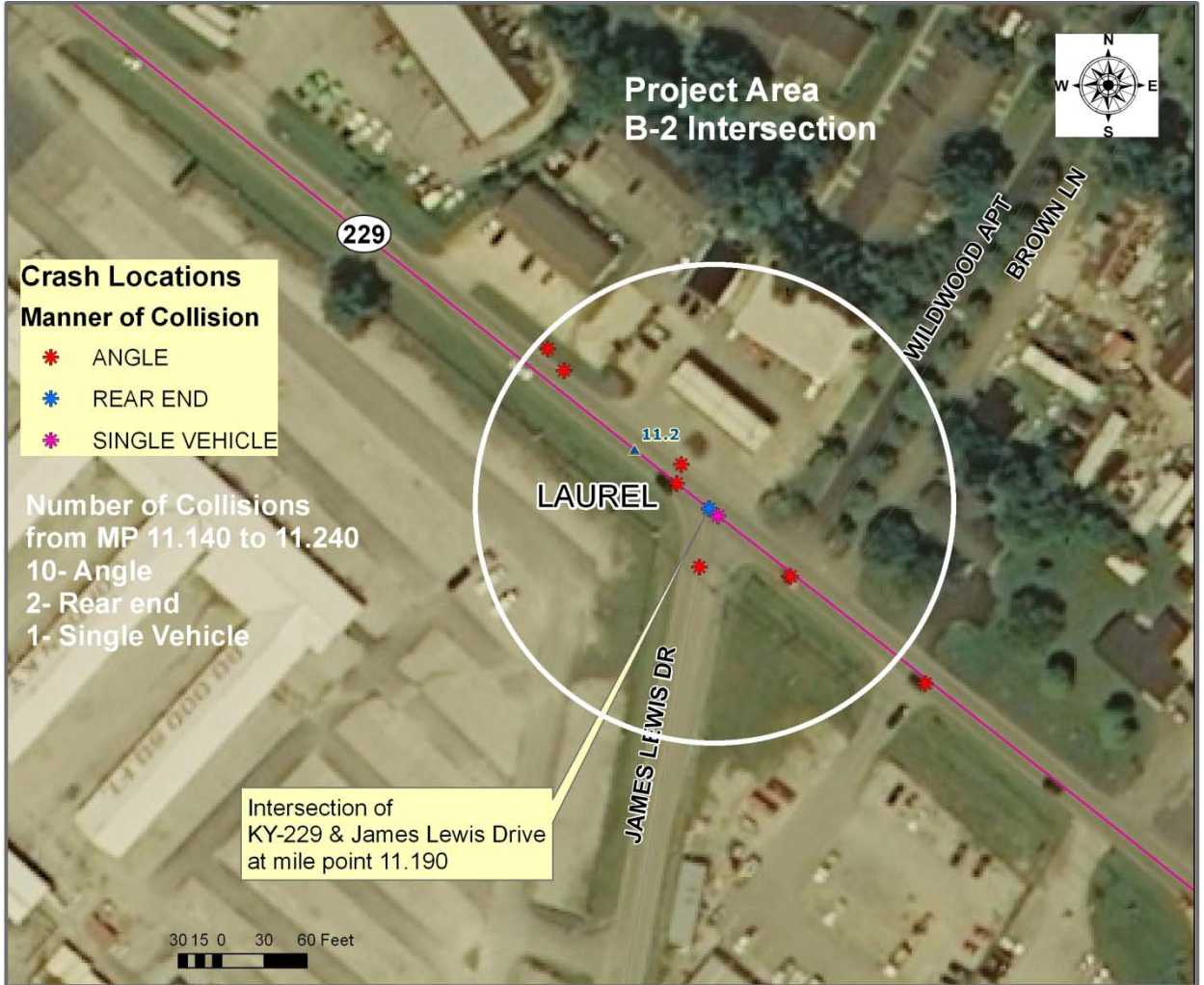
Figure III-18: Section 4- KY-229 High CRF Collision Locations (from MP 11.140 to MP 11.240)
