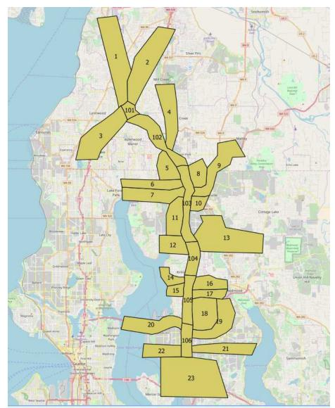
Zones labeled 101-106 are used to filter the trips. For example a trip from Zone 3 to Zone 20 is of no interest if it does not pass through the corridor of interest and can be filtered out.
