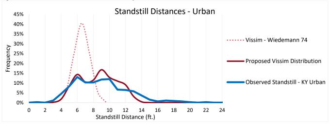
\*Vissim version 11 and onward can apply multiple distributions for standstill distance through the implementation of modifications to the W74 driving behavior and vehicle class compositions. Previous versions of Vissim are limited to singular average standstill distance values with the aforementioned set standard deviation.
