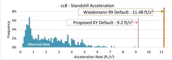
Figure 18: Standstill Acceleration – Observed, Default, and Recommended
