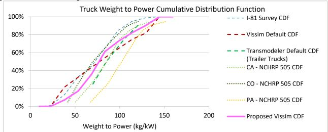
Figure 14: Recommended Weight-to-Power Distribution
