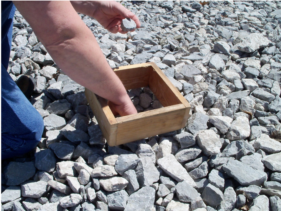
Template used to sample larger aggregate that is not easily shoveled
