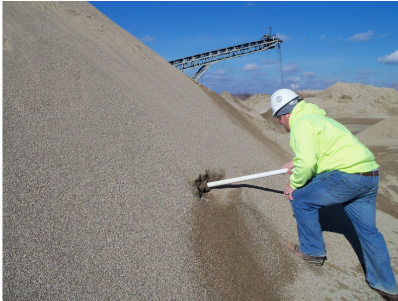
Using a Sand Tube for Natural Sand
