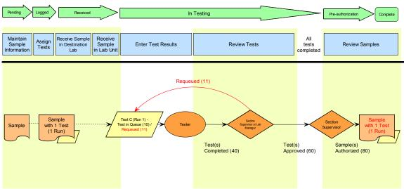
Figure 5-4. Requeue Test Workflow
