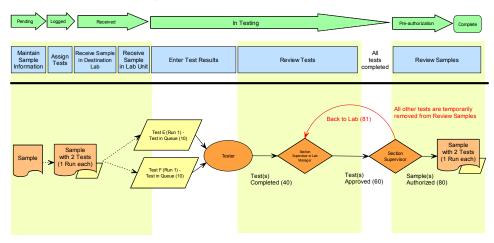
Figure 7-7. Send Test Back to Lab Workflow
