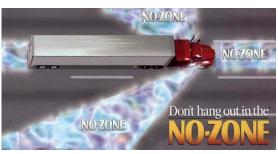
Because of the size, commercial vehicles have large blind spots on both sides. If you cannot see the driver's face in the truck's side-view mirror, the driver cannot see you.
