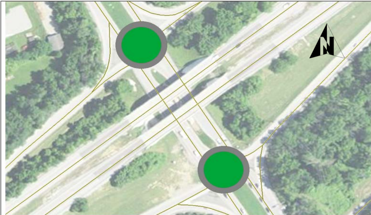
Sizing and location of 130' diameter roundabouts. (Does not include details on approaches and ramps.)
