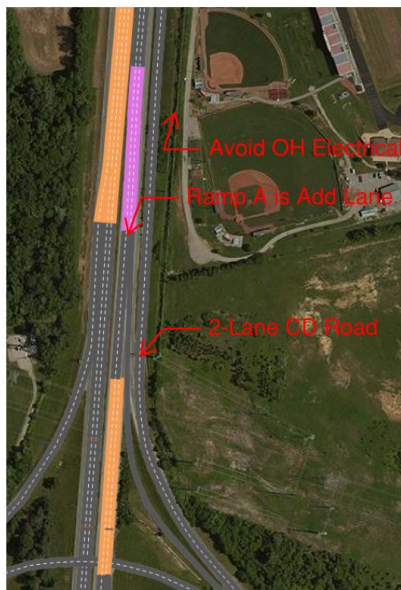
CD Road at Ramp A Merge
