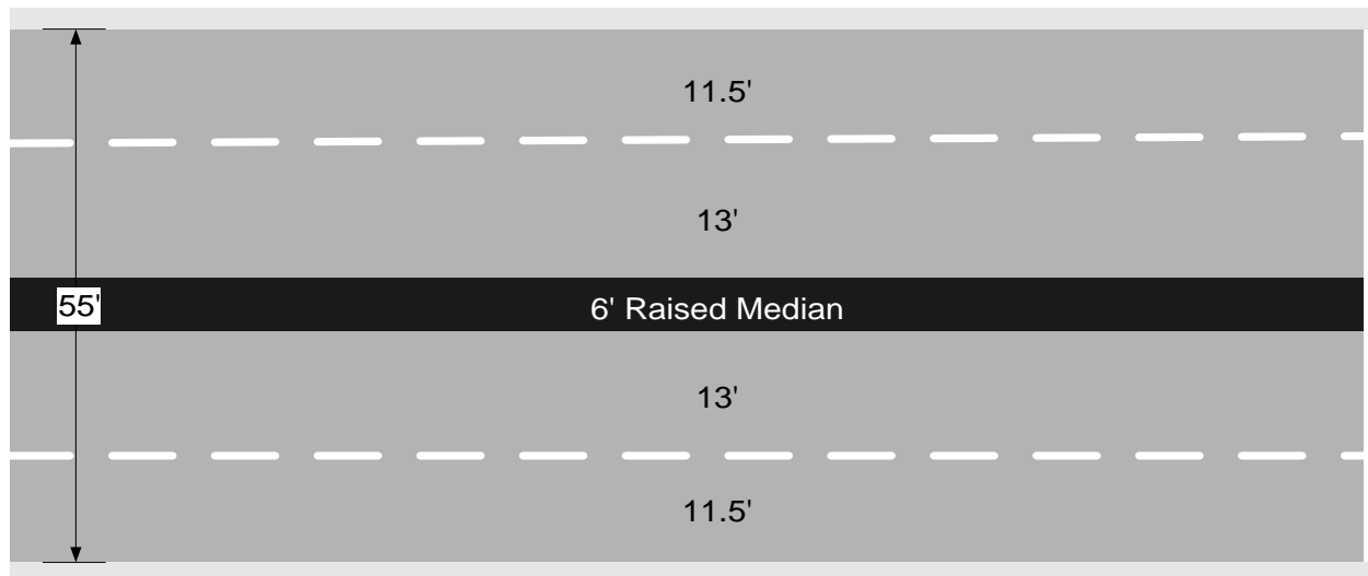
4 lanes with raised median
