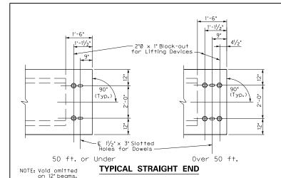
2"Ø x 1" Block-out for Lifting Devices
