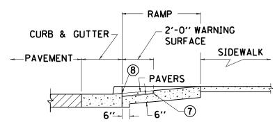
TYPICAL CONCRETE PAVER DETECTABLE WARNING INSTALLATION
