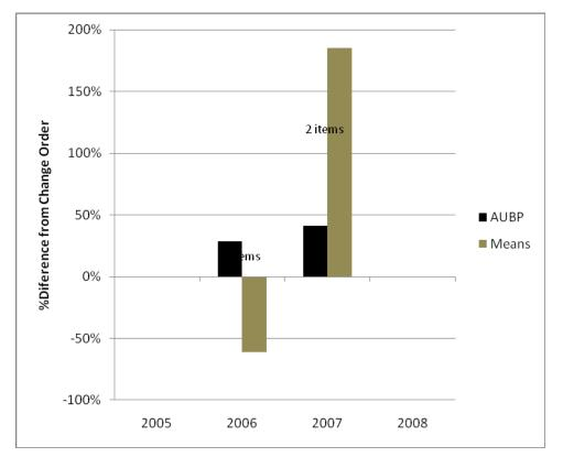
Figure L. 13 Average % Difference between approved change order cost and estimated cost using Average Unit Bid Price (AUBP) and Means for Removing Guardrail End Treatment
