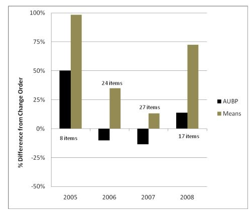
Figure L. 15 Average % Difference between approved change order cost and estimated cost using Average Unit Bid Price (AUBP) and Means for Asphalt Mix for Pavement Wedge
