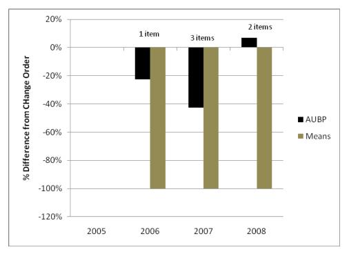
Figure L. 11 Average % Difference between approved change order cost and estimated cost using Average Unit Bid Price (AUBP) and Means for Relocating Crash Cushions
