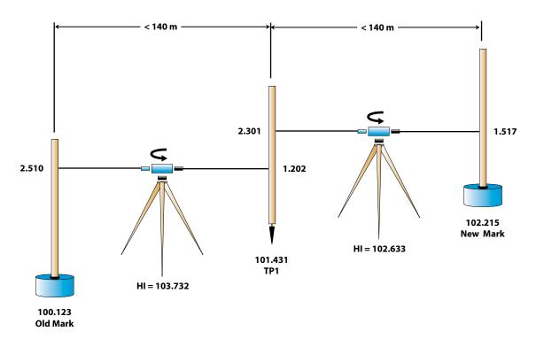
**8.** Compute the elevation of the new point, either the new bench mark or the turning point; this is the difference of the HI (computed in Step 5) minus the foresight.
