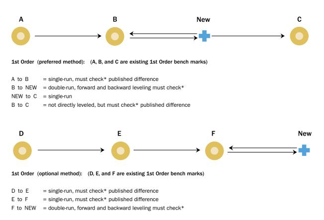
\*Note: "Check" refers to "Maximum section misclosure (millimeters)" of  $4 \times \sqrt{D}$ , as defined for 1st Order, Class II levels; where D is shortest length of section (one-way) in kilometers, in the publication "FGCS Specifications and Procedures to Incorporate Electronic Digital/Bar-Code Leveling Systems."
