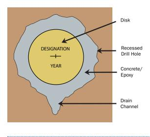
Figure B - 4. Top view of disk in outcrop.
