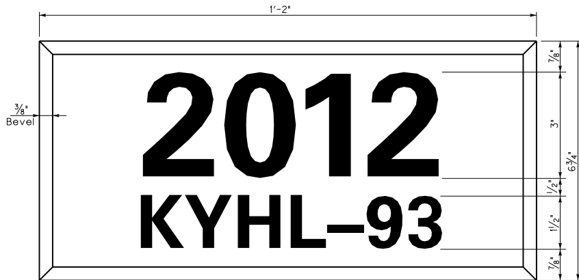
STENCIL FOR YEAR AND DESIGN LOADING When year only is used place year in center of plate
