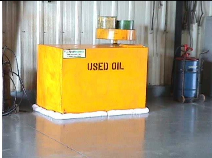
This used oil tank is stored indoors, clearly labeled and the work area is orderly.
