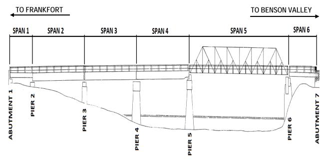
Figure 1: Elevation of the Broadway Bridge with span and substructure numbering.
