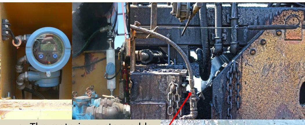
The metering system adds the emulsion based upon the mix design using a Mass Flow Meter.
