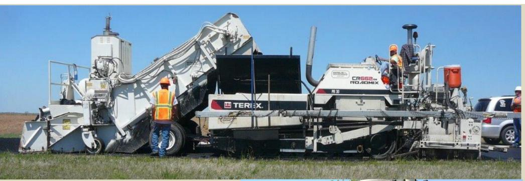
Dustrol uses a paver equipped with two counter-rotating augers that re-blend the material as it is delivered to the screed. This significantly helps reduce segregation of material.
