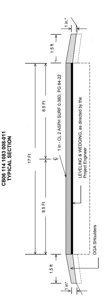
\*Edge of pavement to be tapered using the Durable Pavement Edge Shoe attachment \*Where Existing Site Conditions Permit
