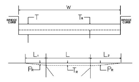
W = bridge width curb to curbT = thickness of existing bituminous overlayL = length of bridge $L_1 \& L_2$  = length of approach pavement to be removedT $T_R$  = thickness to be removed and replaced on bridge $P_R$  = thickness to be removed and replaced on pavementNote:  $L_1 \& L_2$  lengths shall be determined by using a transition rate of 100 ft / inch of thickness
