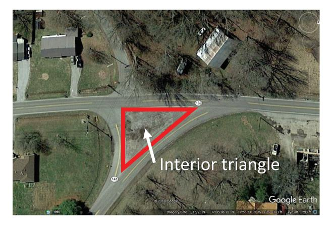
Contractor is to remove all material contained within what shall be referred to as the "interior triangle" as shown above to a depth of approximately 10 inches. The type of material within the interior triangle is unknown. If during the excavation of the interior triangle the contractor finds earth suitable to grow vegetation, the contractor is to leave the earth piled on the right of way for use by District 2 maintenance personnel. This shall be paid for per cubic yard of Roadway Excavation.
