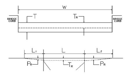
W = bridge width curb to curbT = thickness of existing bituminous overlayL = length of bridge $L_1 \& L_2$  = length of approach pavement to be removed $P_R$  = thickness to be removed and replaced on pridge $P_R$  = thickness to be removed and replaced on pavementNote:  $L_1 \& L_2$  lengths shall be determined by using a transition rate of 100 ft / inch of thickness
