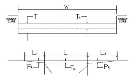
W = bridge width curb to curbT = thickness of existing bituminous overlayL = length of bridge $L_1 \& L_2$  = length of approach pavement to be removedT $T_R$  = thickness to be removed and replaced on bridge $P_R$  = thickness to be removed and replaced on pavementNote:  $L_1 \& L_2$  lengths shall be determined by using a transition rate of 100 ft / inch of thickness
