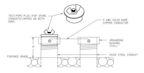
TEST/PIPE PLUG(FOR SPARE CONDUITS) AND GROUNDING DETAIL
