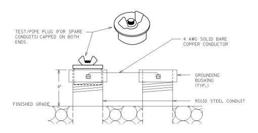
TEST/PIPE PLUG(FOR SPARE CONDUITS) AND GROUNDING DETAIL
