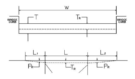
W = bridge width curb to curbT = thickness of existing bituminous overlayL = length of bridge $L_1 \& L_2$  = length of approach pavement to be removed $P_R$  = thickness to be removed and replaced on bridge $P_R$  = thickness to be removed and replaced on pavementNote:  $L_1 \& L_2$  lengths shall be determined by using a transition rate of 100 ft / inch of thickness
