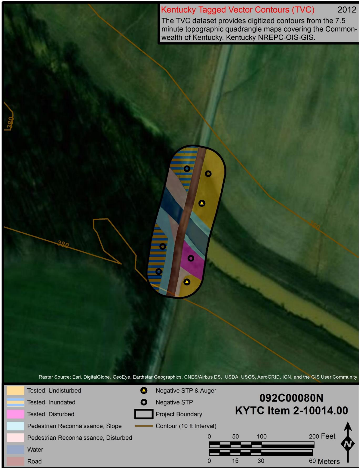
Figure 30. Bridge No. 092C00080N (Item No.2-10014) showing project area conditions and excavated test locations on aerial map.
