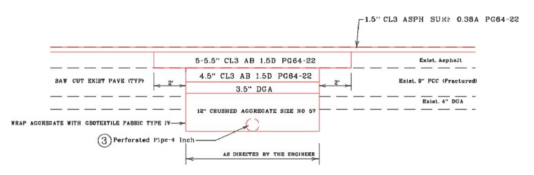
NOTE: Contractor must complete the Base Failure Repairs and open to traffic for a minimum of 7 days before beginning the 1.5" Milling and placing of 1.5" surface part of the contract.
