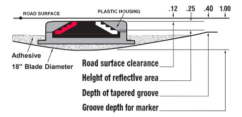
**D. Location and Spacing.** Install the markers in the pattern for high reflectivity with two (2) IPMs per groove. Locate and space markers as shown in the current Standard Drawings or Sepias. (Note: use Inlaid Pavement Markers wherever Type V Pavement Markers are
