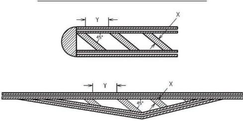
The cross-hatch pavement marking width (X) and spacing (Y) will usually be specified in the plans. The width to spacing values usually have a ratio of 1:10. If the plans do not specify the width (X) and spacing (Y) the Engineer will provide the contractor with the X and Y values for each cross-hatch installation. If necessary, the Engineer may obtain guidance from the District Traffic Engineer and/or the Division of Traffic Operations.
