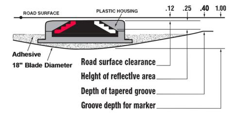
**D.** Location and Spacing. Install the markers in the pattern for high reflectivity with two (2) IPMs per groove. Locate and space markers as shown in the current Standard Drawings or Sepias. (Note: use Inlaid Pavement Markers wherever Type V Pavement
