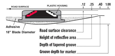
**D. Location and Spacing.** Install the markers in the pattern for high reflectivity with two (2) IPMs per groove. Locate and space markers as shown in the current standard drawings or sepias (note: use Inlaid Pavement Markers wherever Type V Pavement Markers are called for). Do not install markers on bridge decks. Do not install a marker on
