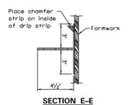
(For concrete deck prior to concrete placement)
