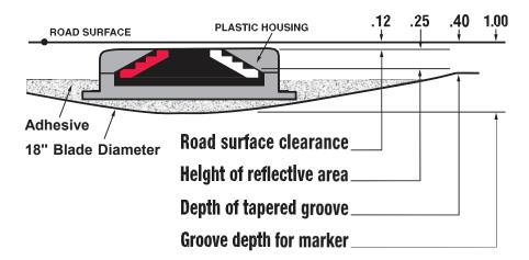
**D. Location and Spacing.** Install the markers in the pattern for high reflectivity with two (2) IPMs per groove. Locate and space markers as shown in the current standard drawings or sepias (note: use Inlaid Pavement Markers wherever Type V Pavement Markers are called for). Do not install markers on bridge decks. Do not install a marker
