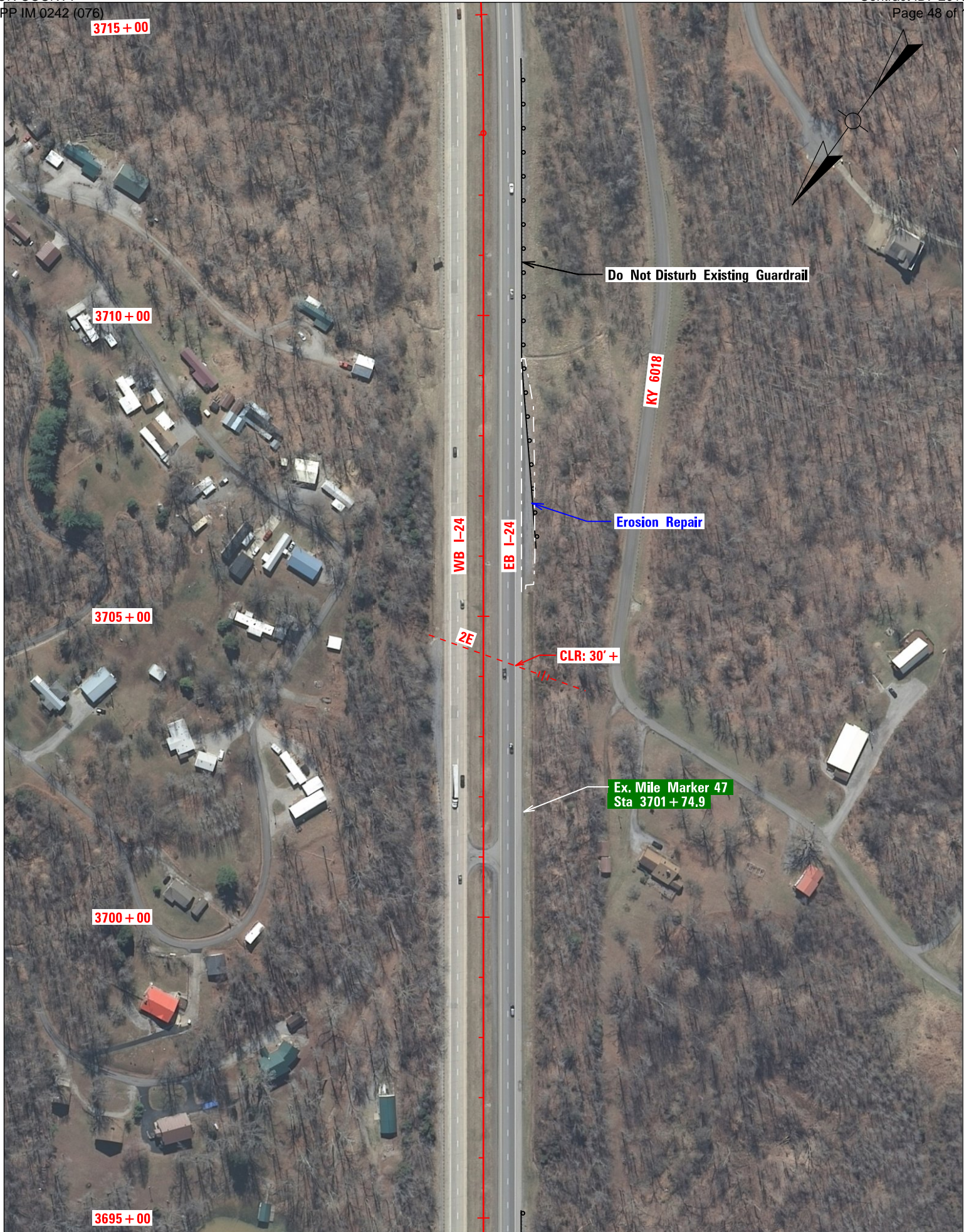
Eastbound I-24 Rehab Plan - Scale 1" = 200' - Sheet 6 of 19 - Sta 3695+00 To Sta 3715+00
