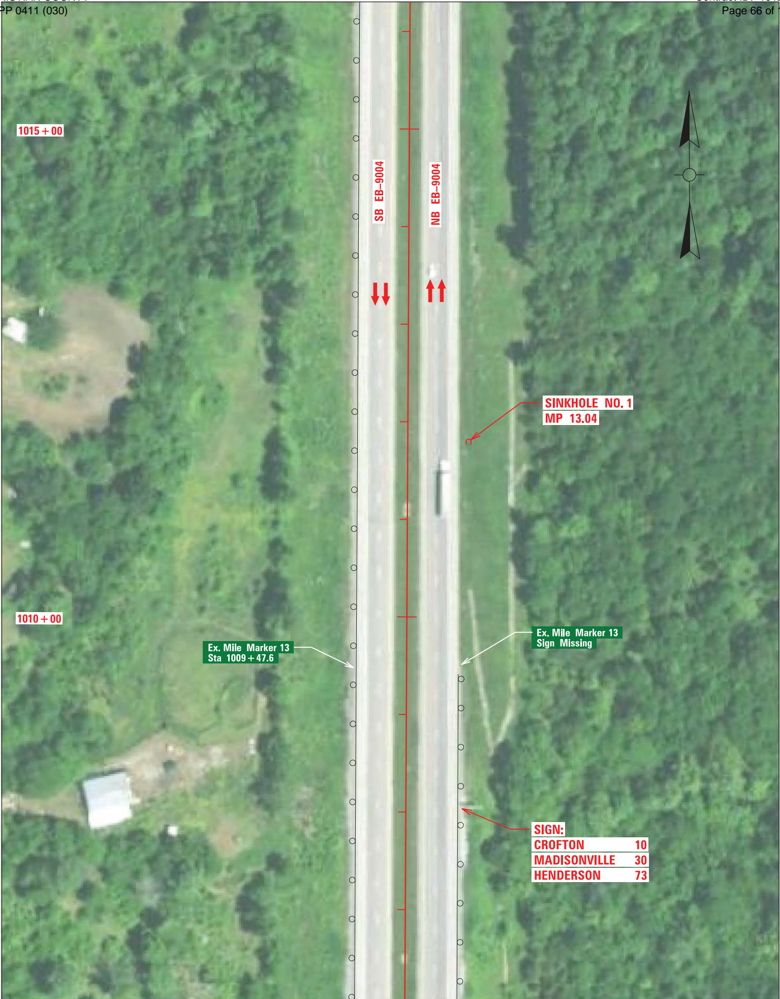
EB 9004 Rehab - Sinkhole No. 1 - MP 13.04 - Scale 1" = 100'
