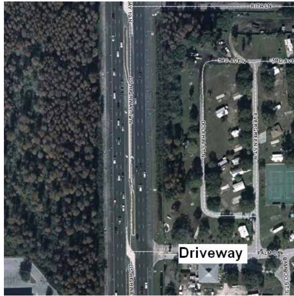
Figure 4-7 Aerial Photograph of a Sample Site Which Accommodates U-turns at a Median Opening
