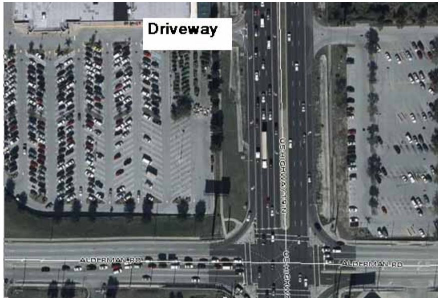
Figure 4-8 Aerial Photograph of a Sample Site Which Accommodates U-turns at a Signalized Intersection
