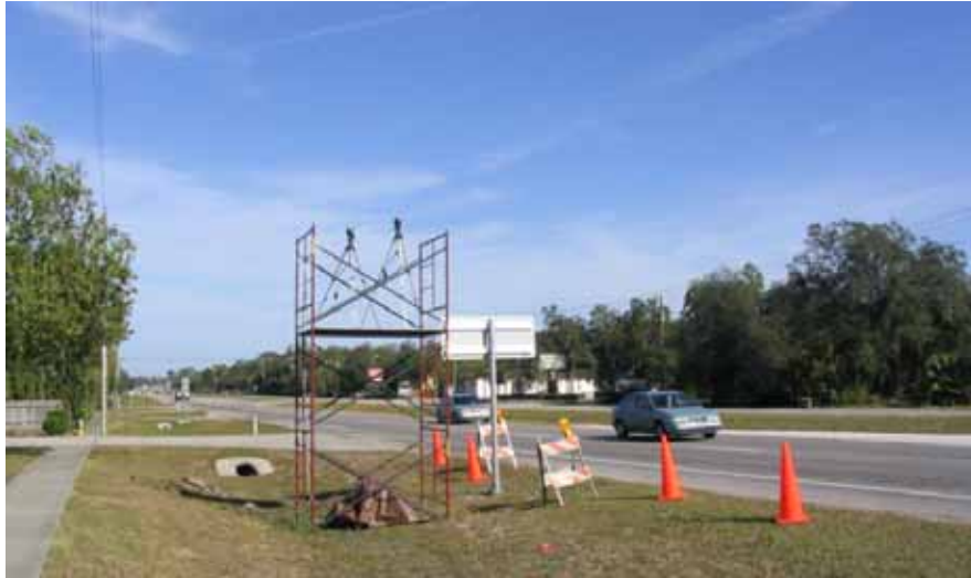
Figure 4-1 Video Cameras Set Up On Scaffolding
