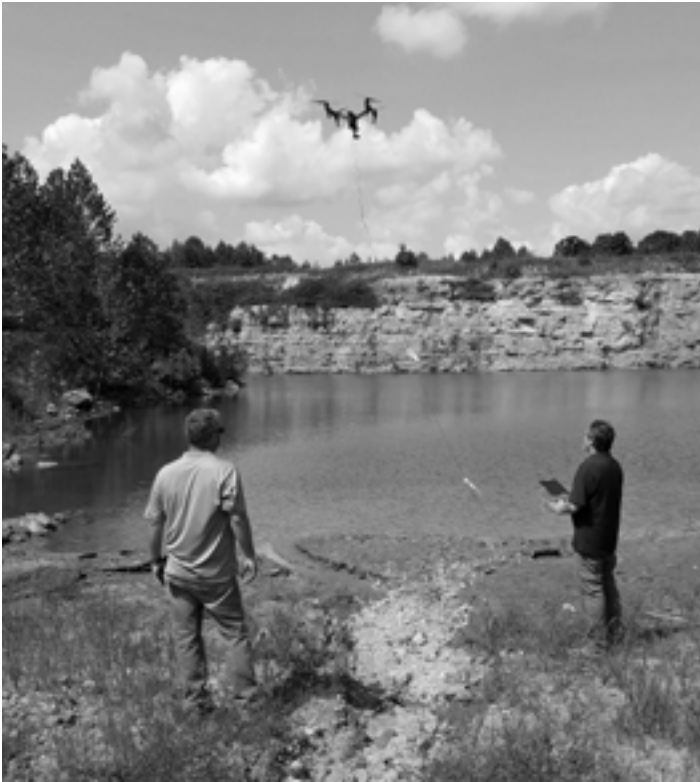
Robert Cammack and Adam Humphrey of Kentucky's Energy and Environment Cabinet, use a drone to estimate the volume of water in a mining pond.
