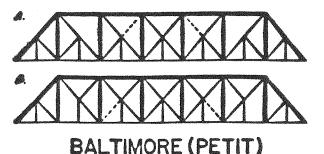
IB71- EARLY LOTH CENTURY A. A PRATT WITH SUB-STRUTS. B. A PRATT WITH SUB-TIES. LENGTH: 250-600 FEET \$6-180 METERS
