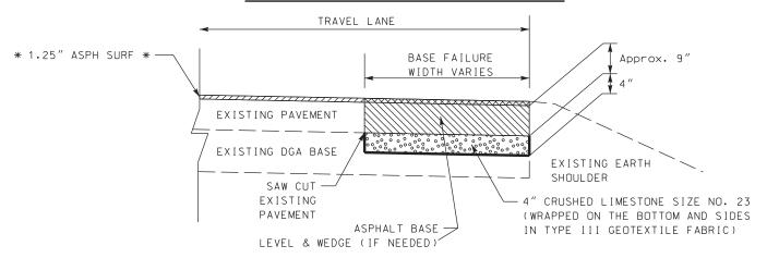
\* For Base Failure Repair locations within the limits of Resurfacing/Overlay Sections # 1 & 2, Overlay the Base Failure Repair with 1.25" Asph Surf. according of the Special Notes. For Base Failure Repair locations outside of the Resurfacing Limits, Mill & Inlay 1.25" Asph Surf according to the "Profile" and "Top View" details below, and according to the Special Notes.
