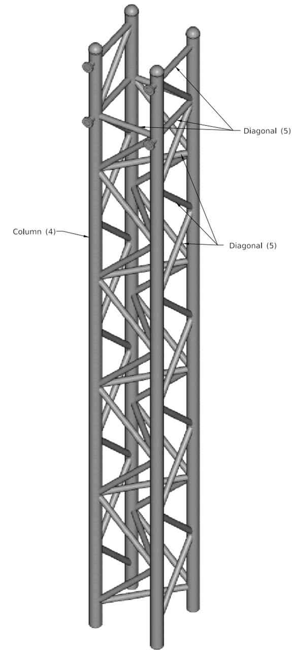
**ISOMETRIC VIEW OF CANTILEVER COLUMN**
