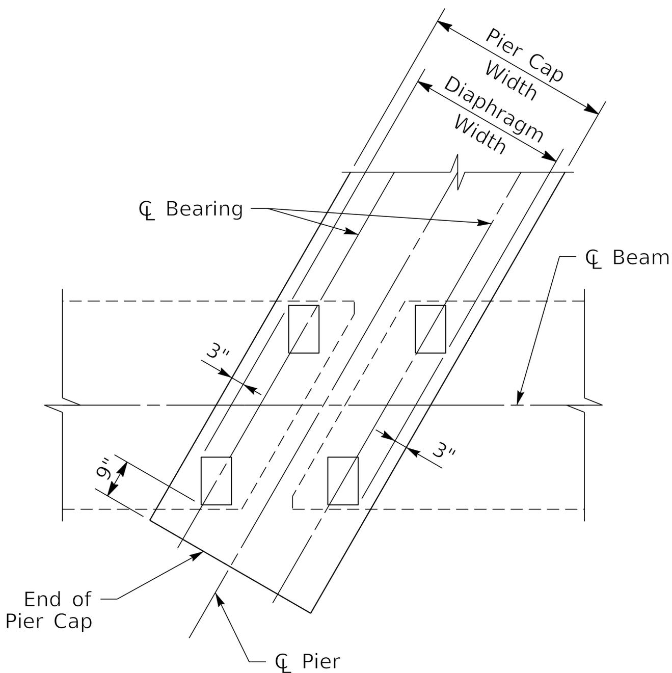
Dimensions shown to pad edges are minimums. Take care to ensure beams are not overhanging pier caps excessively when single pads are used under beams with large bottom flange widths. The Division of Structural Design reserves the right to require larger dimensions than those shown
