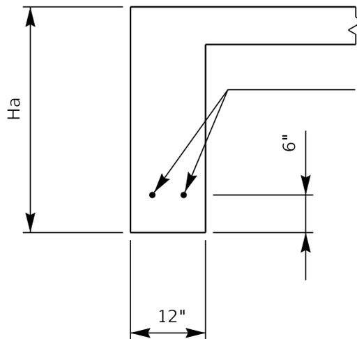
Use two bars same size as N bars in multiple span culverts. In single span culverts use two bars the same size as A bars.
