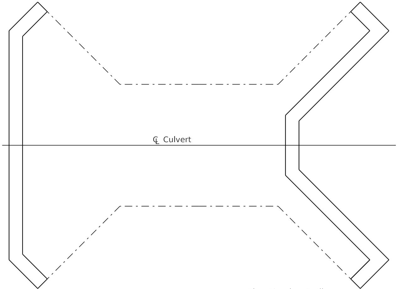
Plan Showing Outline of Apron for Culverts with Paved Inlet/Outlet
