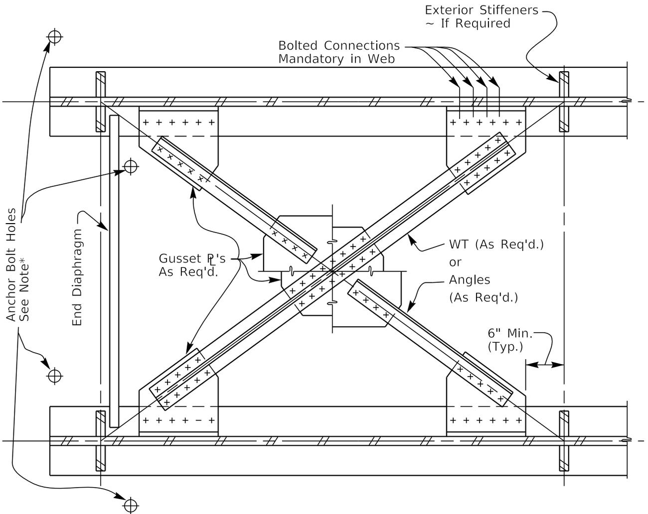
Fasteners shown are for illustration only. WT's may be welded to Gussets
