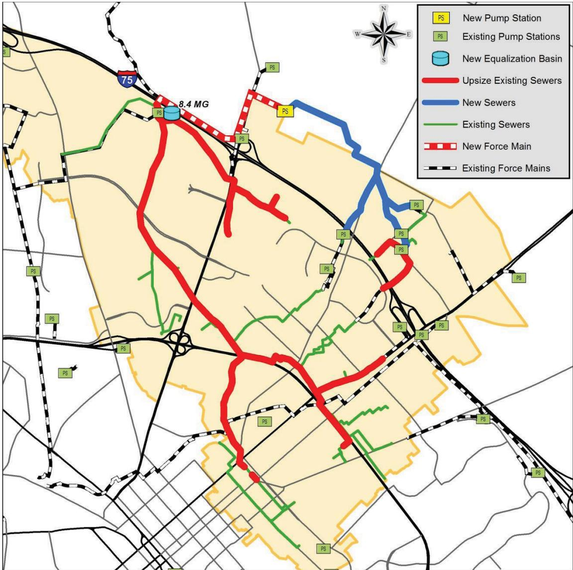
Figure 3-3: Localized Storage General Solution – Cane Run
