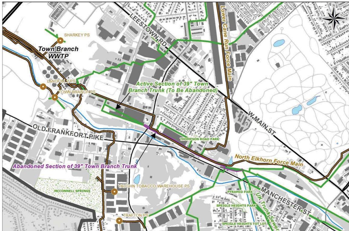
**Town Branch Pump Station Replacement** - The Town Branch Pump Station is identified as an SSO in Appendix A of the Consent Decree and was evaluated as part of the Pump Station Design, Capacity, and Equipment Adequacy Evaluation. Based on this evaluation and its history of SSOs, LFUCG has elected to replace the existing pump station and force main. RMP improvements are to include replacement of the pump station and force main with sufficient capacity to eliminate SSOs for the established LOC.
