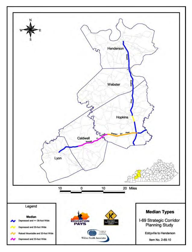
Figure 9. Illustration of Median Types and Widths along Parkways
