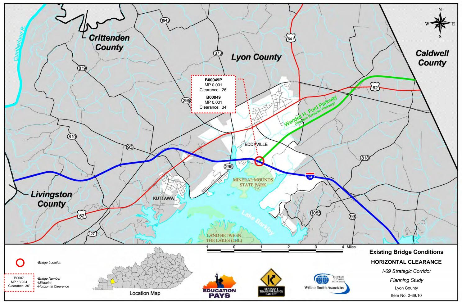
Figure 10. Substandard Horizontal Bridge Clearances for Lyon County 5-5
