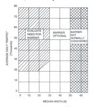
Suggested guidelines for median barriers on high-speed roadways. Figure 6.1 from AASHTO's Roadside Design Guide
