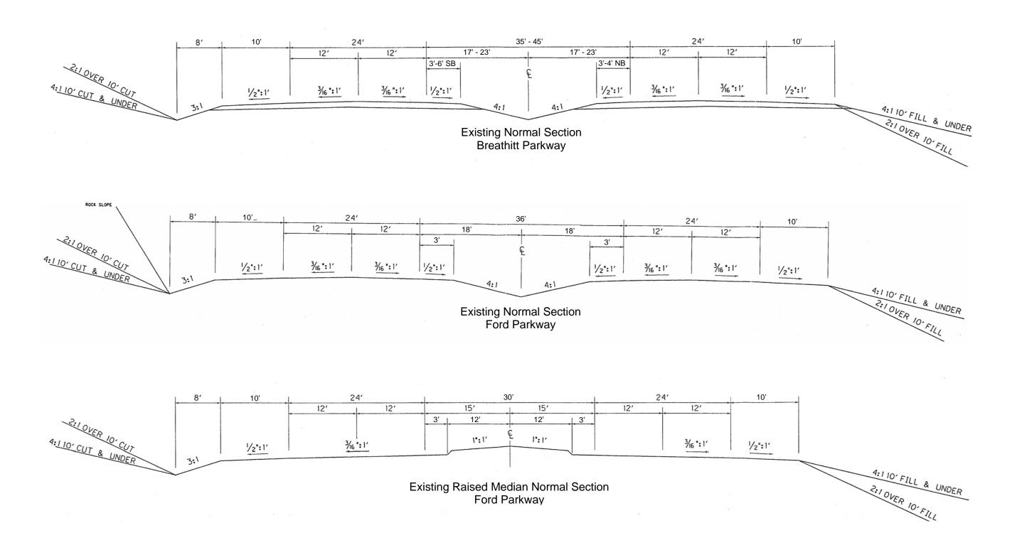
Note: Typical Sections are based upon As-Built Plans provided by the Kentucky Transportation Cabinet.
