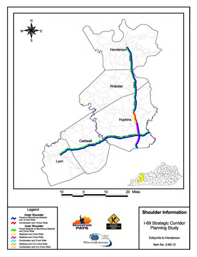
Figure 8. Illustration of Inside and Outside Shoulder Widths along Parkways
