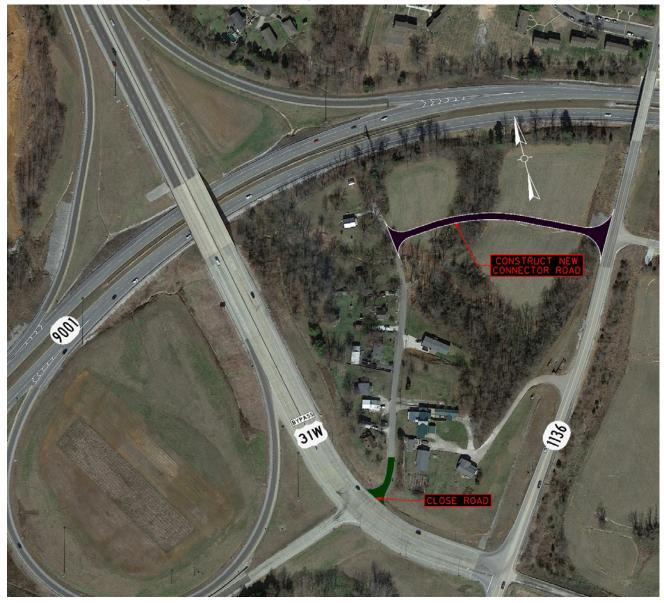
Figure 28: Exit 136, US 31W Bypass Control of Access Improvement
