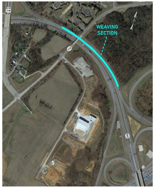
Figure 11: Exit 136 (US 31W) and Exit 137 (I-65) Weaving Section
