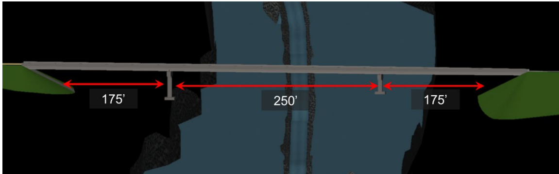
Figure 20: Bridge South of the Ferry
