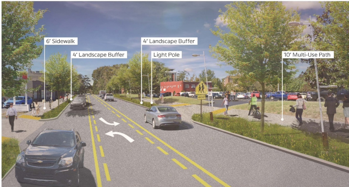
Main Street Improvements with Additional Right-of-Way (60') Proposed Bicycle and Pedestrian Improvement Concepts
