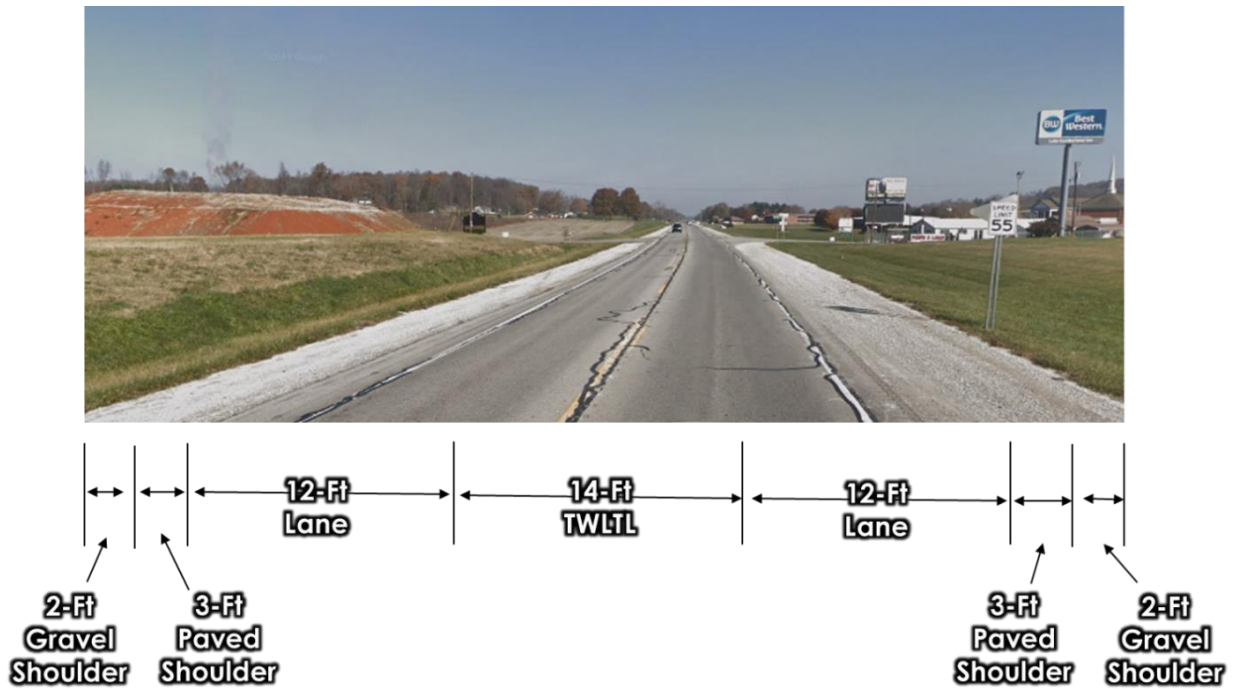
Figure ES-2: TWLTL Typical Section
