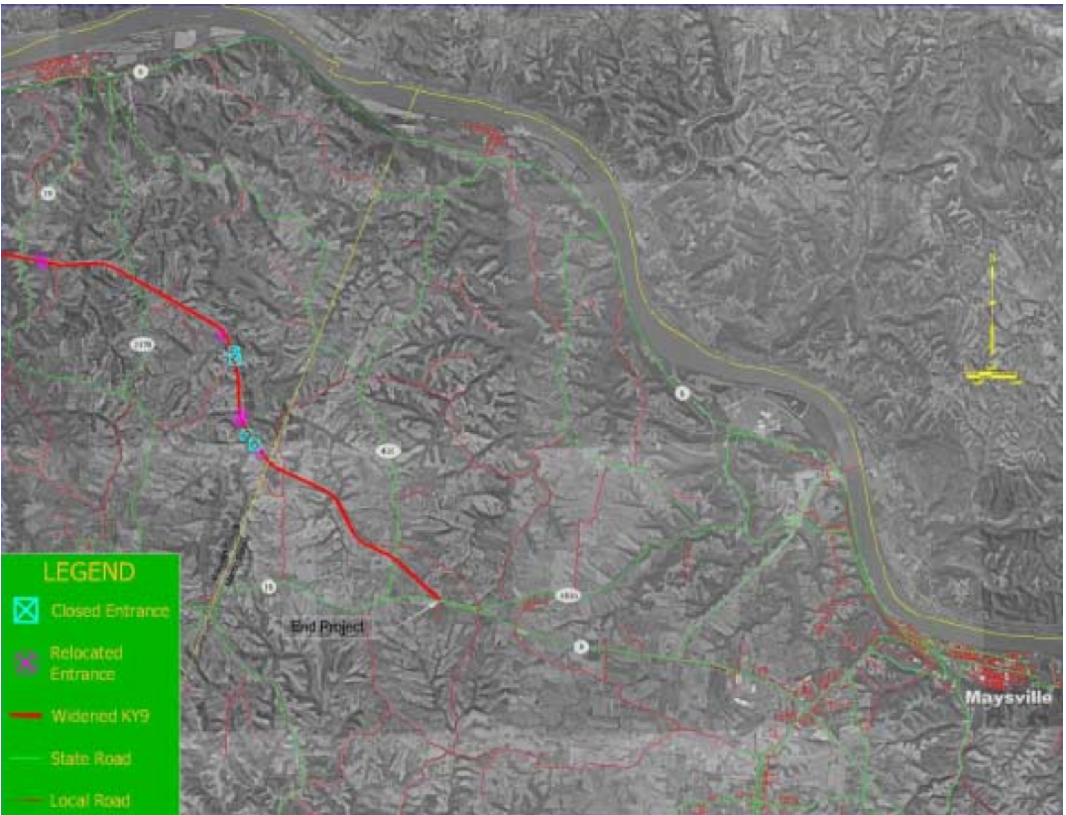
FIGURE 7 – 4-LANE PARTIALLY CONTROLLED ACCESS EAST-SIDE OF CORRIDOR
