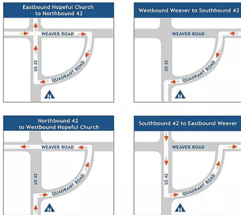
Figure ES-2: New Jug Handle Layout at US 42/KY 842
