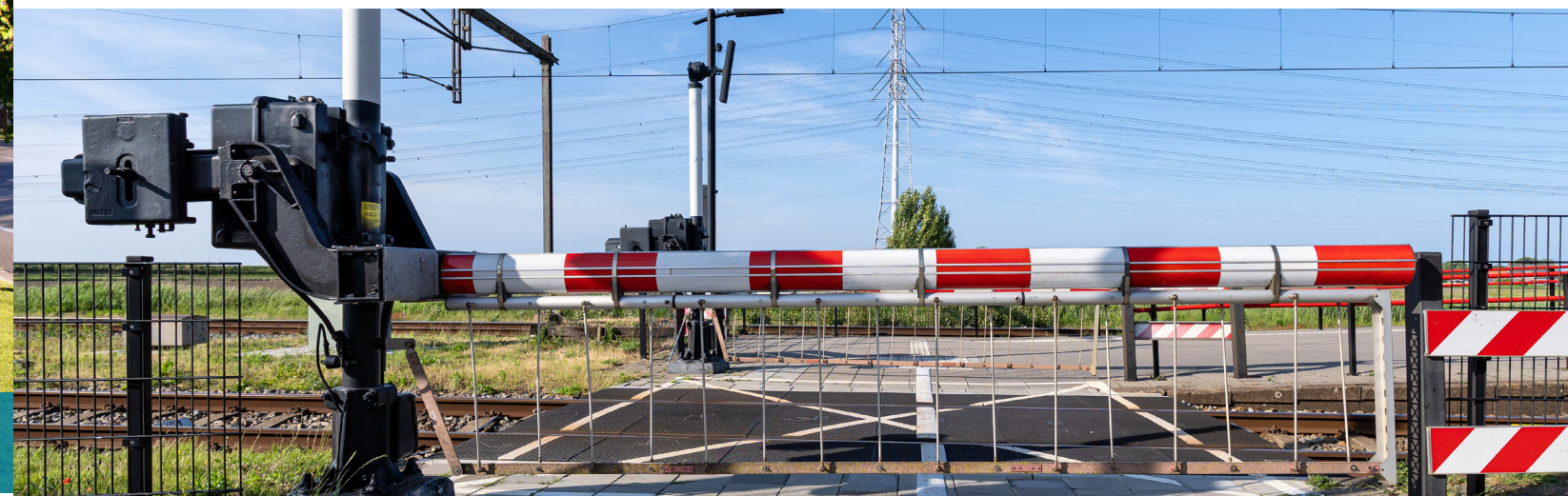
A pedestrian railroad crossing gate can be installed for enhanced safety, along with a defined path.
