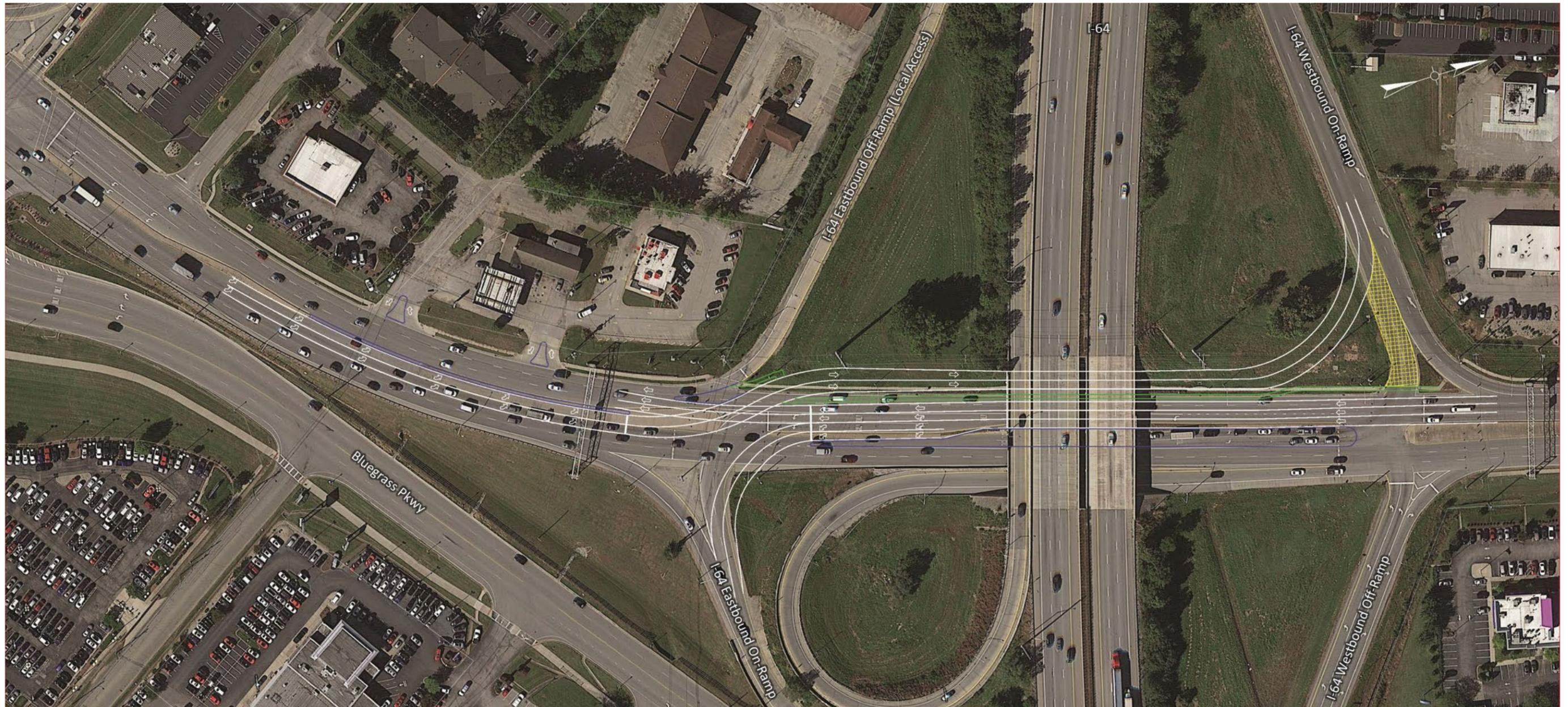
Figure 36: Concept Sketch of Displaced Left Turns
