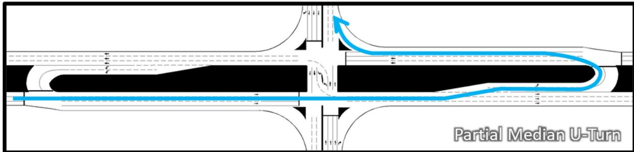
**Figure 46: Left Turn from Cross-Street in Partial Median U-Turn Intersection**
