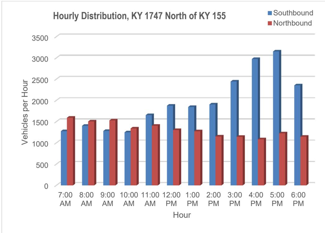
**Figure 16: Hourly Volume Distribution by Direction**
