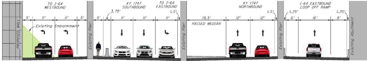
**Figure 35: Typical Section Beneath I-64 Overpass (Looking North)**
