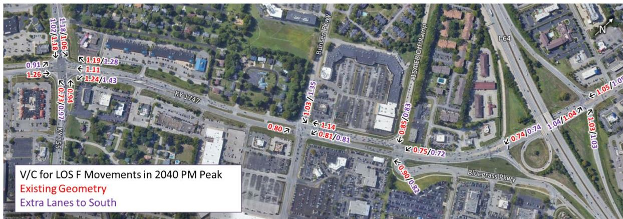
Figure 44: V/C for LOS F Movements, 2040 PM Peak Hour
