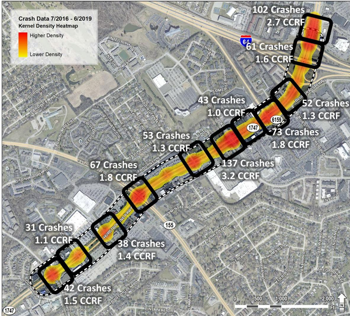
**Figure 24: High CCRF Spots by Crash Density**
