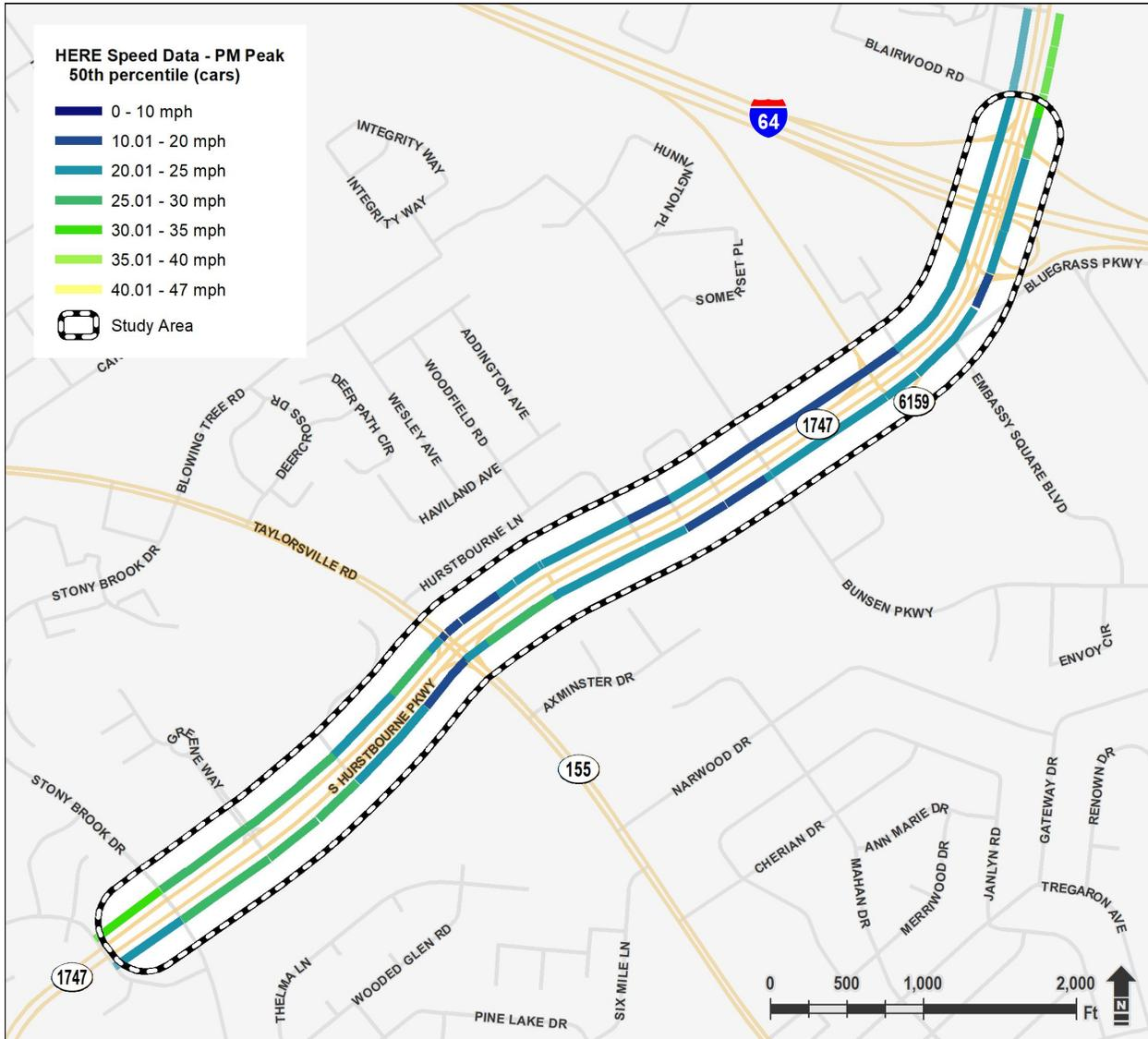
**Figure 9: Observed Travel Speed during PM Peak Period**
