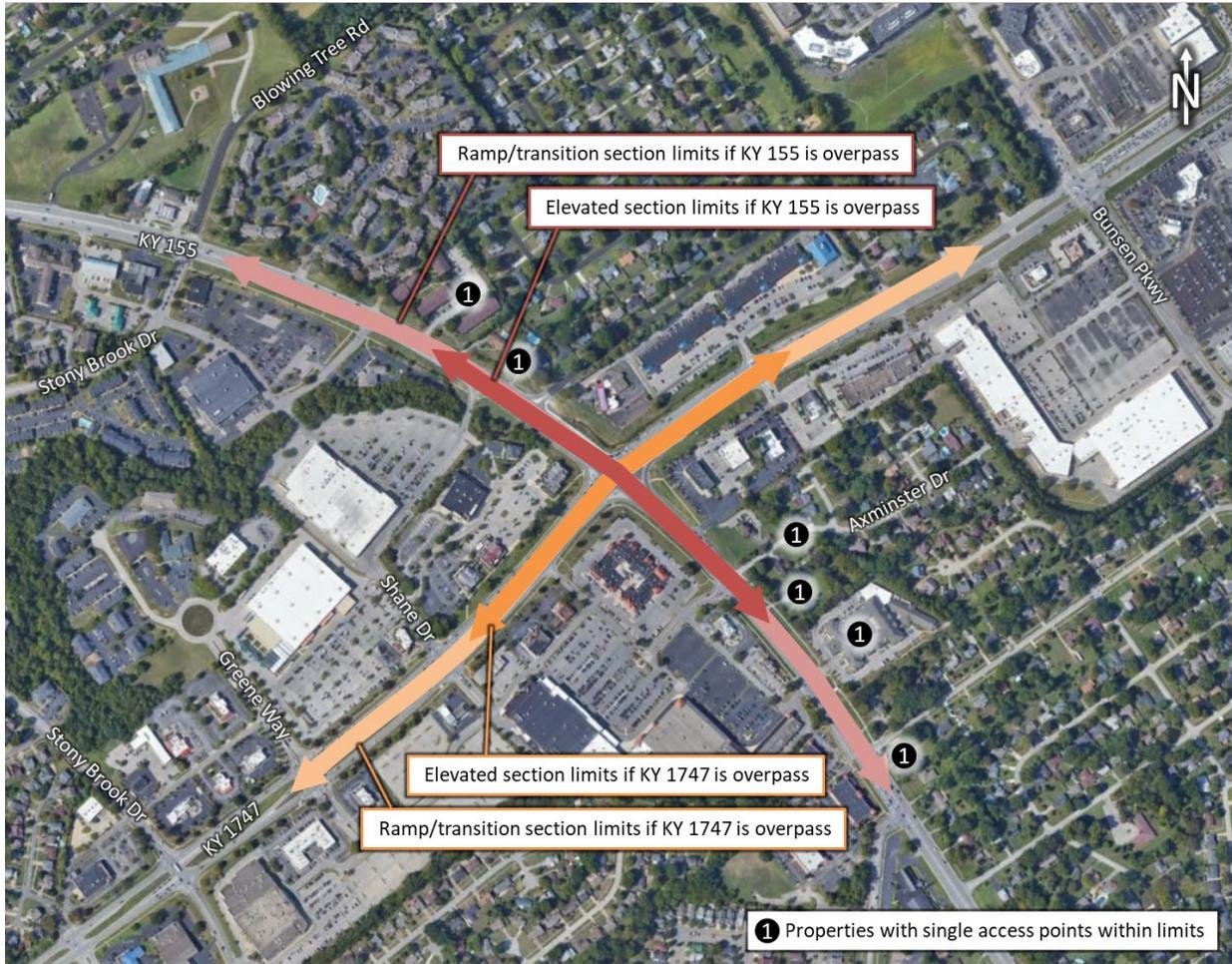
**Figure 47: Elevated Roadway and Transition Lengths for Interchange**
