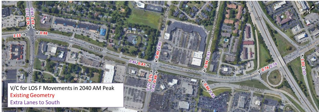
Figure 43: V/C for LOS F Movements, 2040 AM Peak Hour
